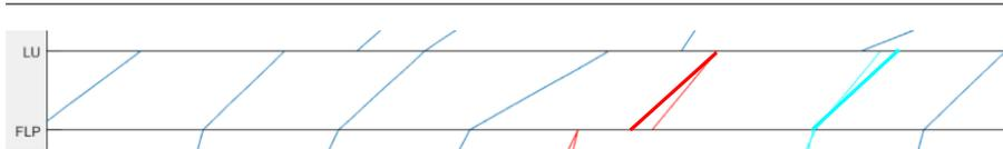
**Fig. 7** Earliest and latest possible train path of the passenger train PX2-2000 and the freight train GR421410 (bold lines) for the bottleneck shown in red and light blue, respectively. All existing trains in the time table are shown in dark blue.
